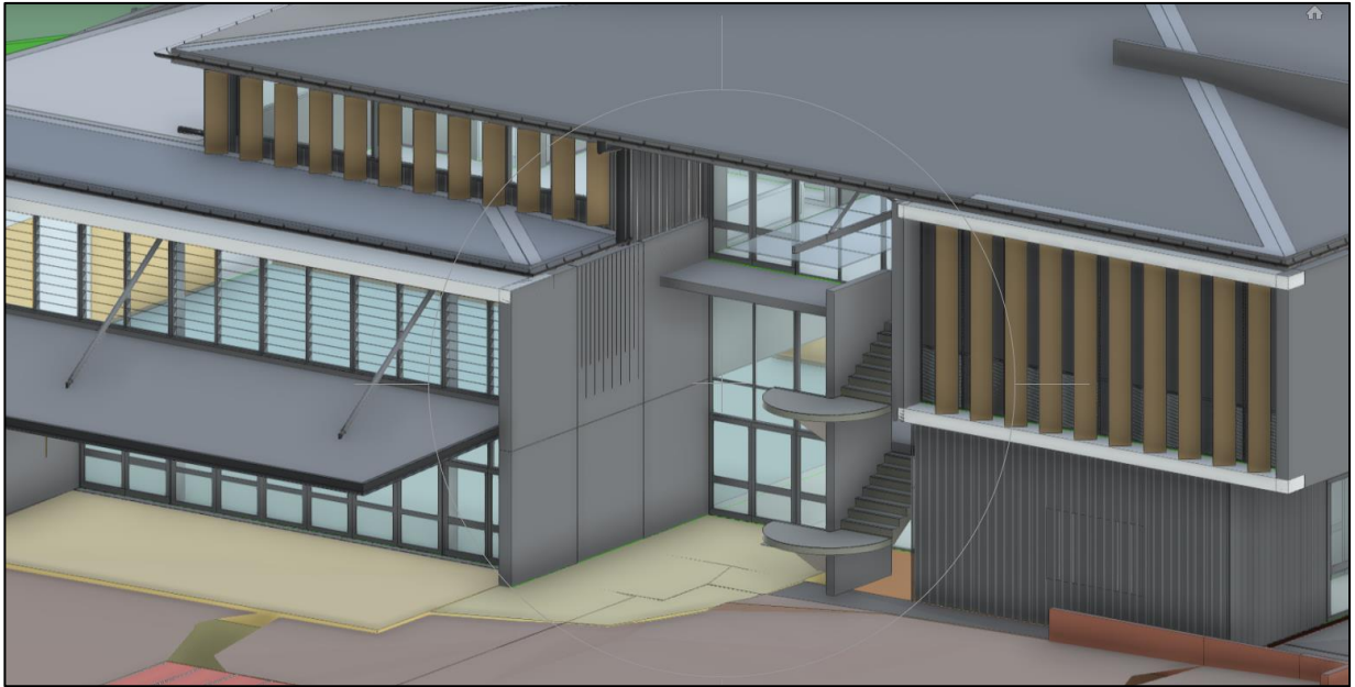
Figure 3 - Indications of shading devices - louvres and awnings - included in the design.
